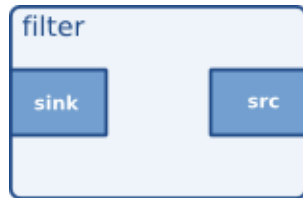
Figure 5-2. Visualisation of a filter element
